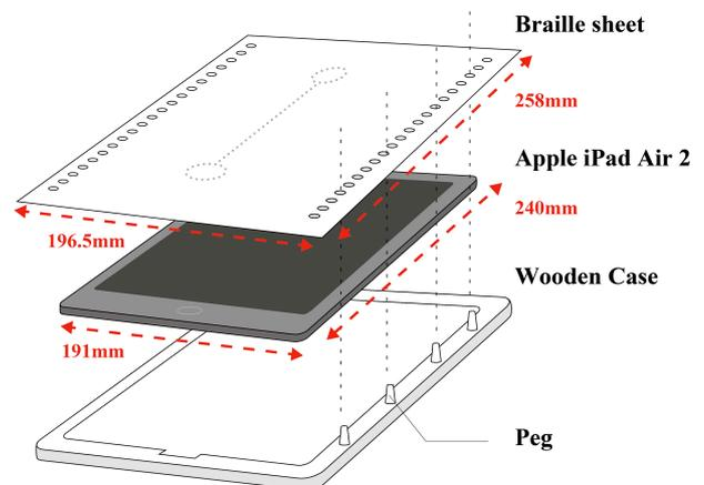
Figure 3: System configuration
