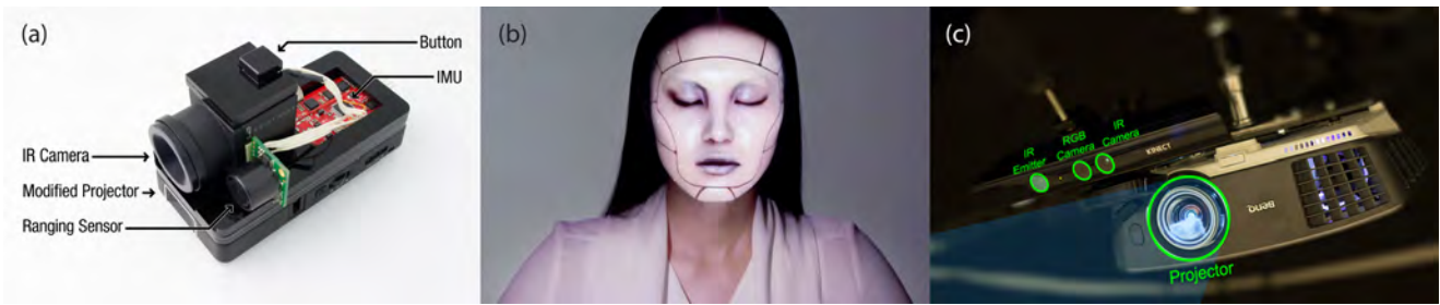
Figure 2 - Dynamic SAR interactions designed for moving supports depend on image sensors to detect target object movements before updating contents to be projected. (a) Side by Side hand-held camera-projector device. (b) Reflective IR markers detected by cameras, used on Project Omote, (c) Scanning the environment with Microsoft Kinect sensor in RoomAlive project.
